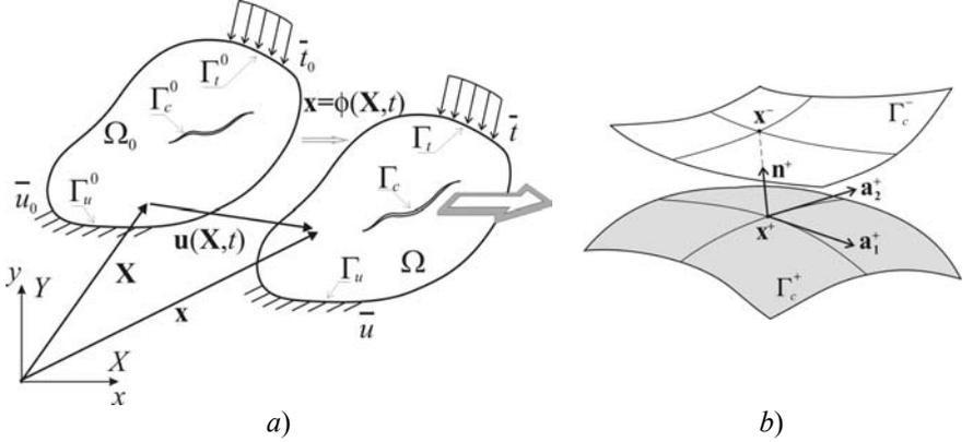
Fig.1. A body with a discontinuity and its representation in the reference and the current domains (a) and zoom of the discontinuity surfaces (b).
