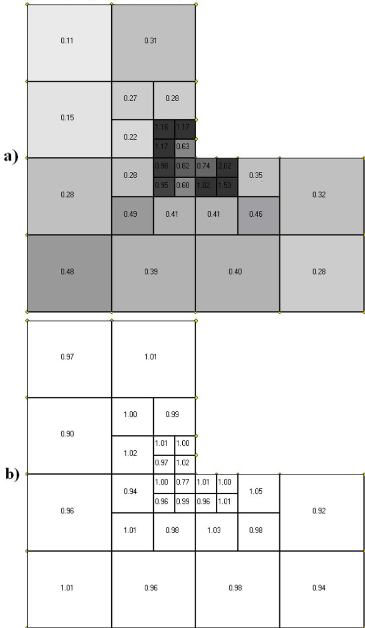
Fig. 6: Nonconforming mesh in Problem B: error estimator  $\eta$  (a), effectivity index  $\theta$  (b).
