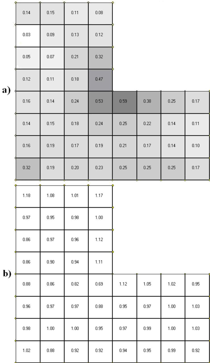
Fig. 5: Conforming mesh in Problem B: error estimator  $\eta$  (a), effectivity index  $\theta$  (b).
