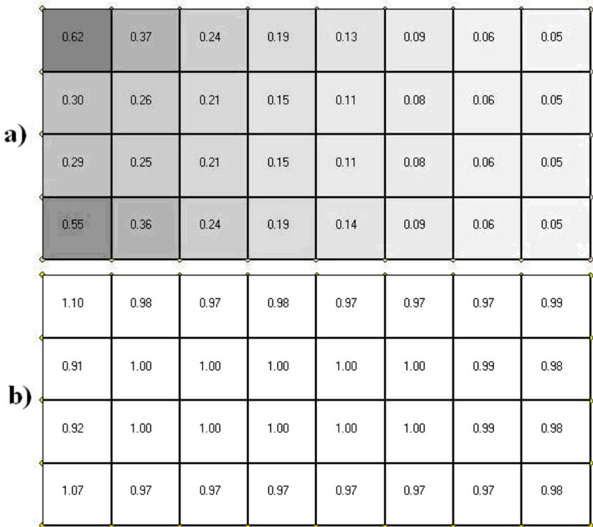
Fig. 3: Conforming mesh in Problem A: error estimator  $\eta$  (a), effectivity index  $\theta$  (b).
