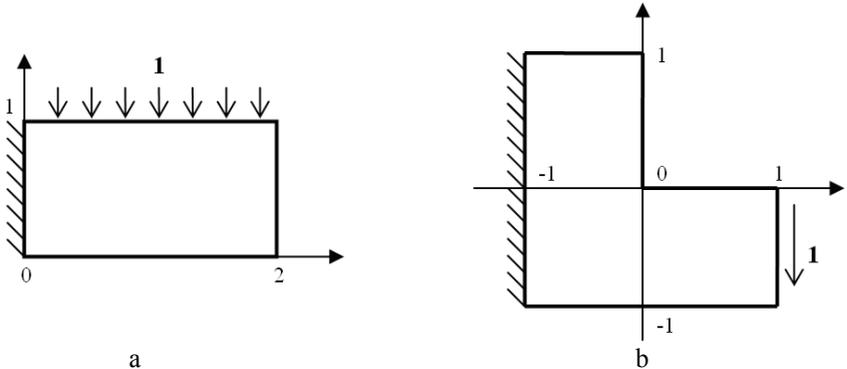
Fig. 2: Geometry and loads of the test problems
