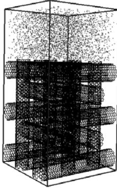
Fig.2. Initial configuration for mutually orthogonal SWNTs array ( $g = 0.3$  nm)
