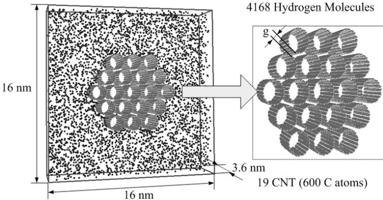
Fig.1. Geometric parameters of the array of SWNTs ( $g = 0.3 \text{ nm}$ )
