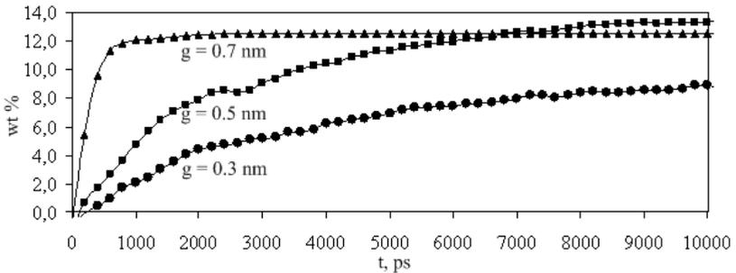
Fig.3. The percentage of adsorbed hydrogen from time for various values of the gap between the tubes
